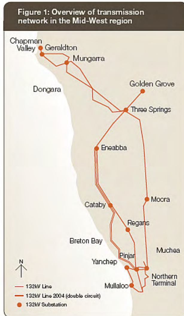
Figure 1: Overview of transmission network in the Mid-West region
